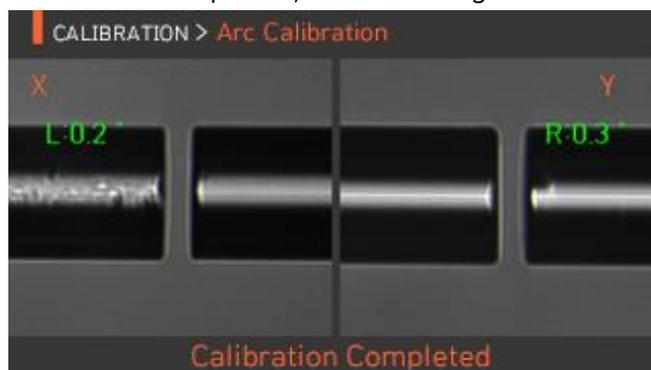
iv. If it is necessary to stop the arc even before the arc calibration is completed, it immediately stops when pressing
